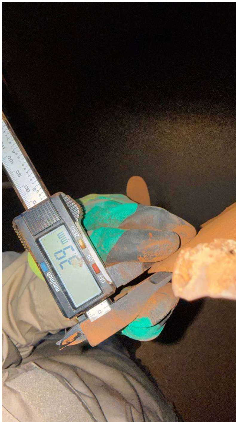
50-rasm. Metall qoplamaning qalinligini o‘lchash jarayoni
