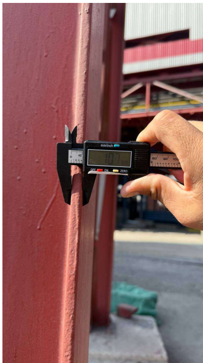
23-rasm. Metall tayanch elementining devor qalinligini o‘lchash jarayoni
