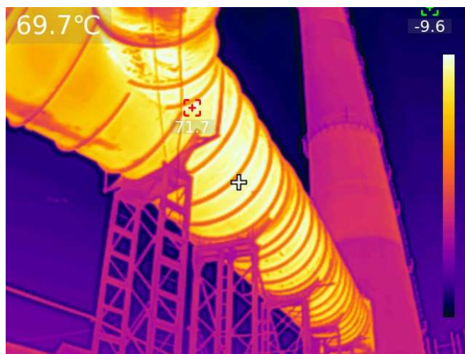
37-rasm. Gaz tozalash tizimidan chiqayotgan gazoxod trubasining termovizor tasviri
