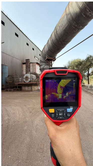
38-rasm. Gazoxod trubasining termovizor yordamida harorat nazoratini o‘tkazish jarayoni
