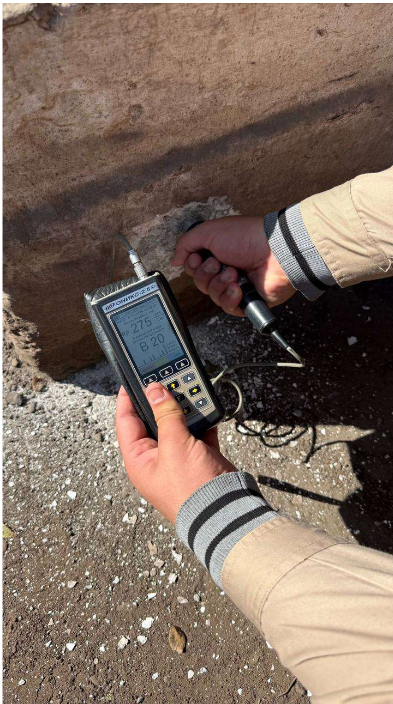
18-rasm. Beton asosning mustahkamlik darajasini aniqlash jarayoni
