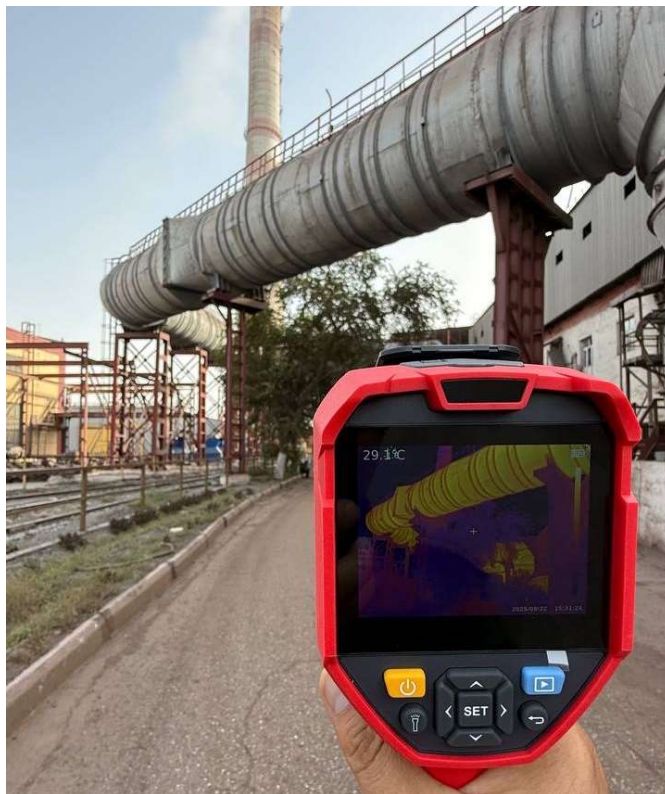
36-rasm. Gazoxod trubasining termografik tekshiruvi
