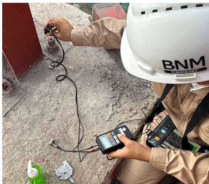
17-rasm. Metall ankerni ultratovush usuli bilan sinovdan o'tkazish jarayoni.
